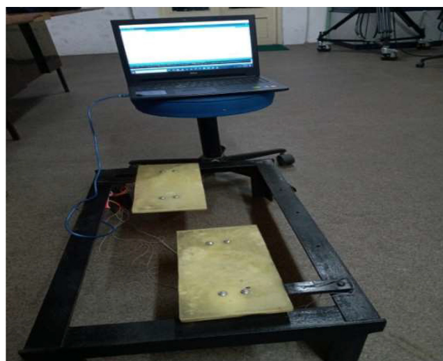
Fig. 2. Force plate test setup.
